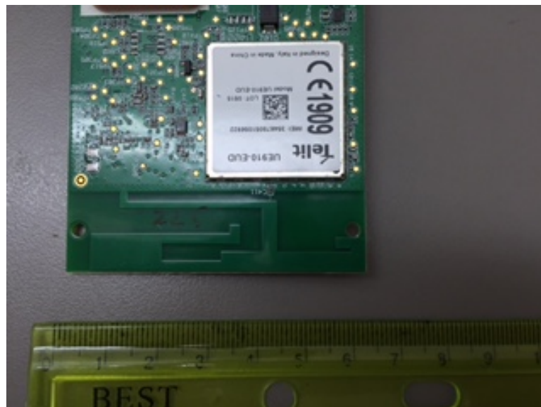
Photograph 11.4.4 Component side of the RF PCB
