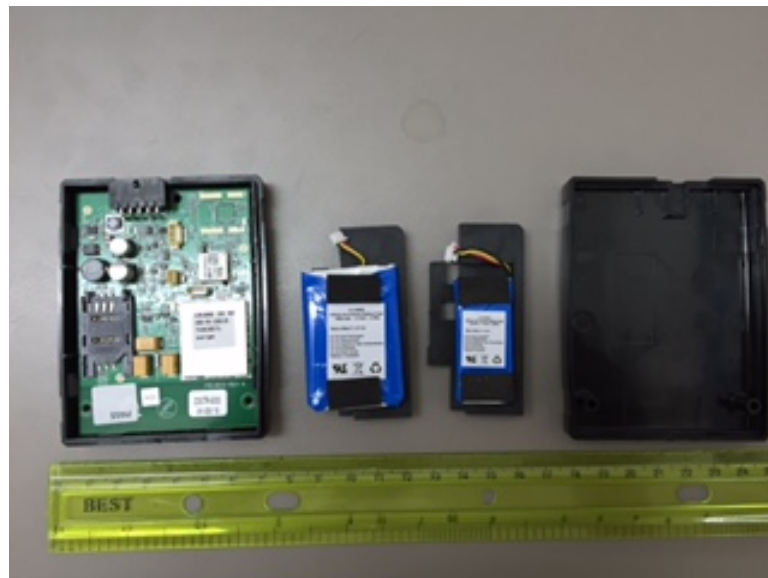
Photograph 11.4.2 Component side of the main PCB
