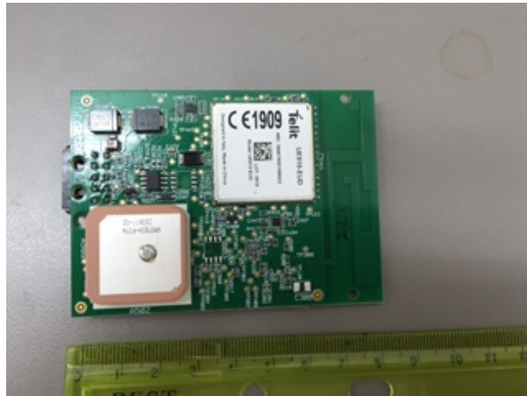
Photograph 11.4.4 Component side of the RF PCB
