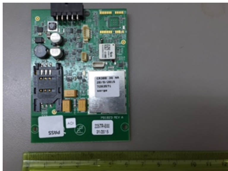
Photograph 11.4.2 Component side of the main PCB
