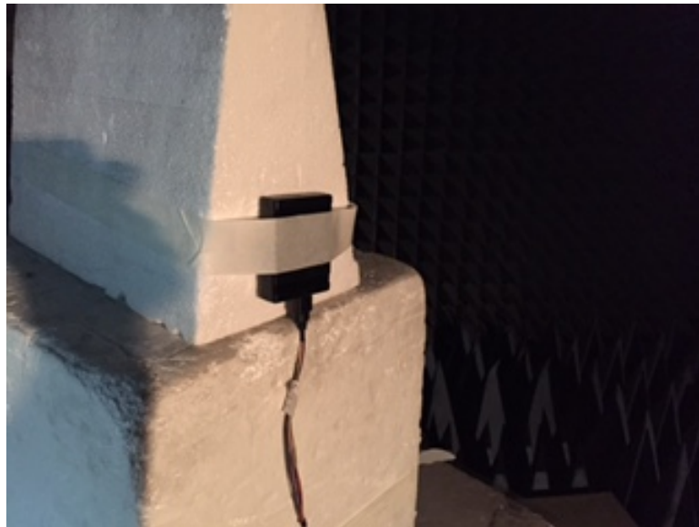
Photograph 6.5.2 EUT in Y-axis orthogonal position
