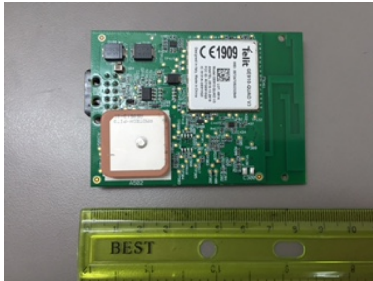
Photograph 11.2.4 Component side of the RF PCB
