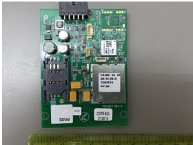
Photograph 11.2.2 Component side of the main PCB
